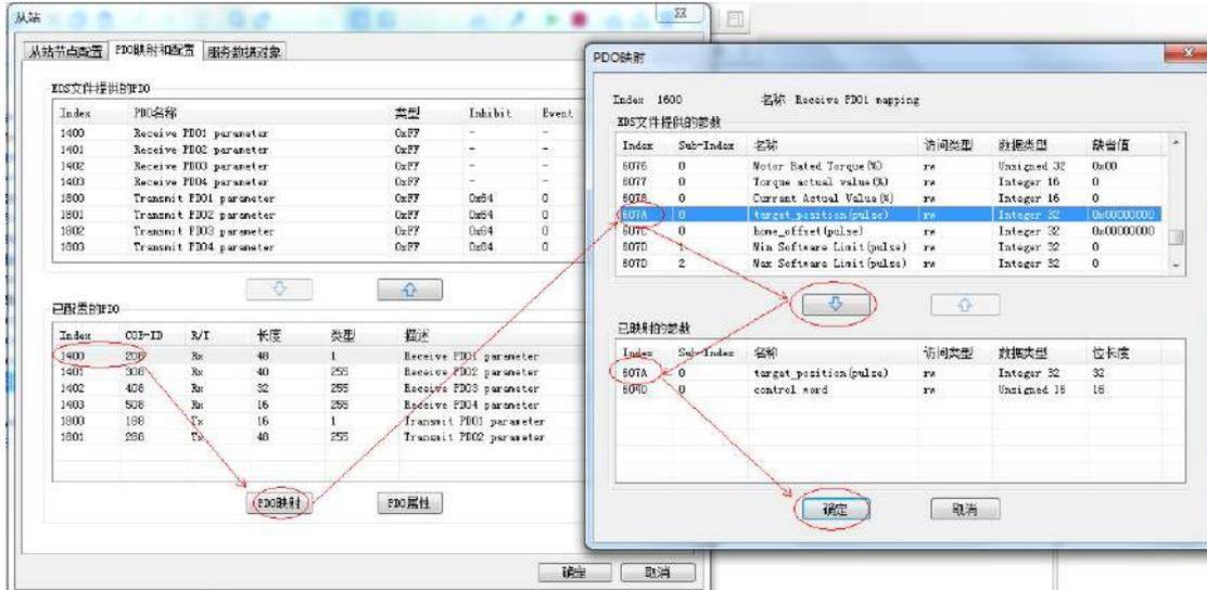
V. select the parameters to be mapped from "parameters provided by EDS file", click the down arrow to add the mapping; select the mapping to be deleted from "mapped parameters", and click the up arrow to remove the mapping, as shown in the following figure:
