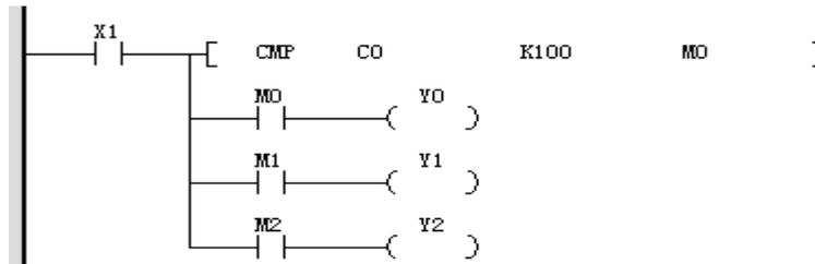
When X1 is ON, C0 is greater than 100, M0 is ON, and Y0 has an output.
