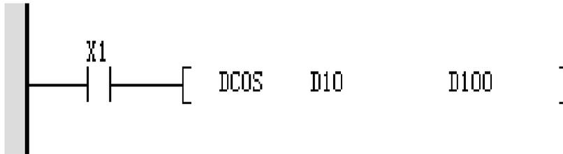
When X1 is ON, the radian (D11, D10) is obtained as the COS value and stored in (D101, D100). The source data and COS result calculated here are in Binary floating number format.
