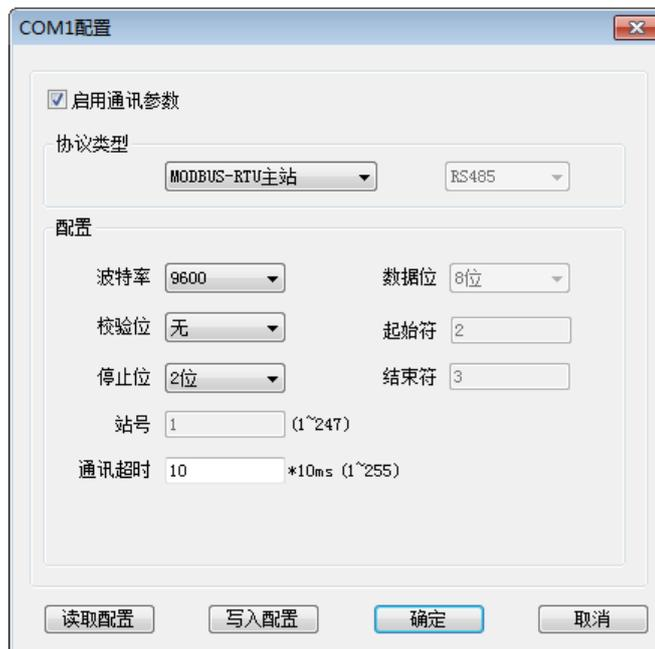
Set as MODBUS-RTU master station, baud rate as 9600, check bit as none, stop bit as 2, station number as 1, communication timeout as 10, click OK after setting.
