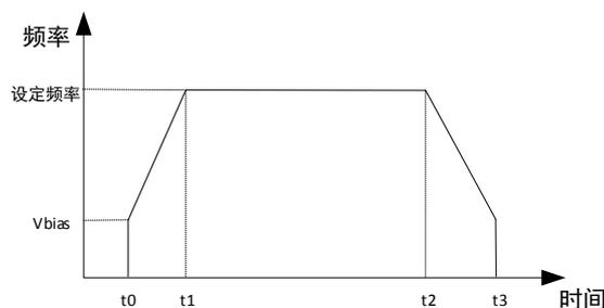
② when the energy flow of the pulse output is off, the pulse output frequency will gradually slow down to the base frequency and then stop the output. Note that in the process of deceleration, when
