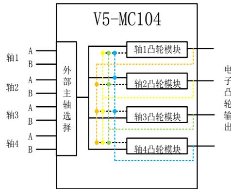
Note: The solid line in the figure selects the external pulse input for the spindle; the dotted line in the figure is the spindle to select the virtual connection.
