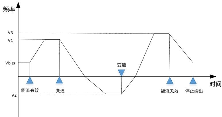
Figure b: Schematic diagram of PLSV2 pulse output change (reverse speed change)
