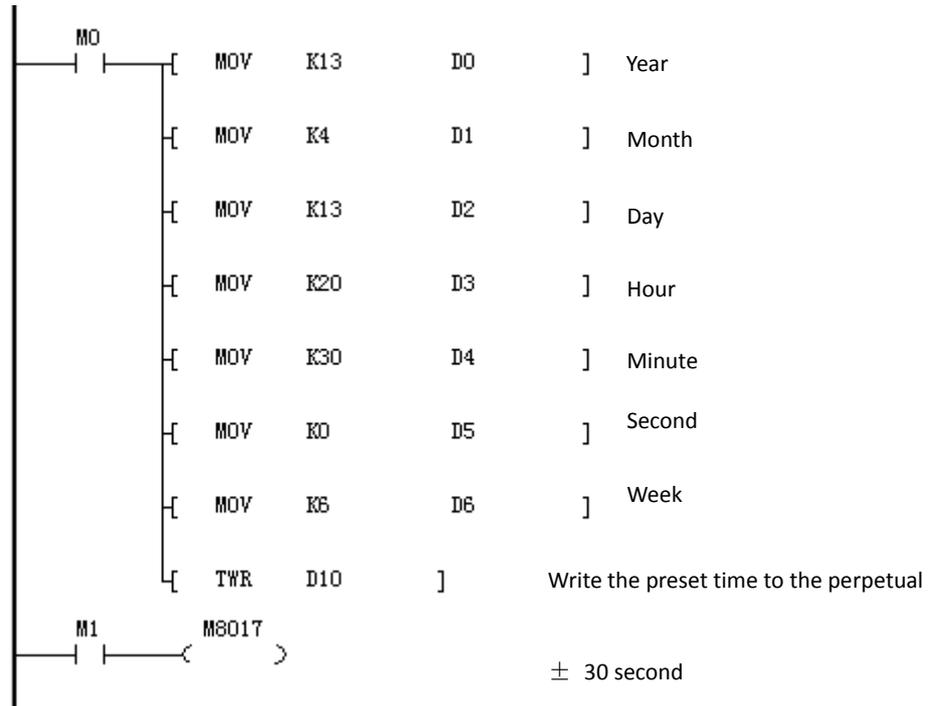
Adjust the current time of PLC to 08:30:00 on April 13, 2013, Saturday; write it to d0-d6 some time in advance, when M0 is set to on, set this time into PLC.
