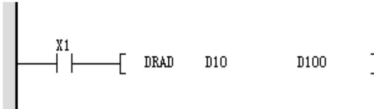
When X1 is ON, the Binary floating number value in (D11, D10) is stored in angle (D101, D100) after the operation is angled to radians.
