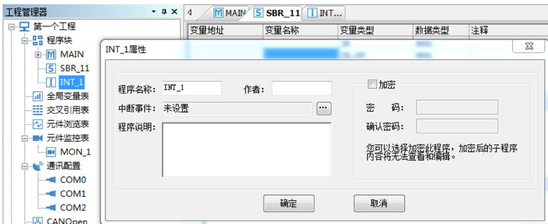
Click the "..." button, the interrupt allocation dialog box will pop up, where the currently available idle interrupts and the interrupts that have been used by other interrupt subroutines are displayed. You can select an interrupt number in the idle interrupt to assign to the current interrupt subroutine, as follows The figure shows:
