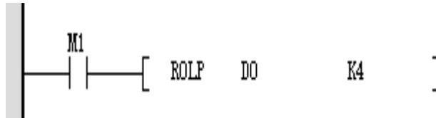
When M1 is on, the number cycle of d0 shifts four bits to the left;
