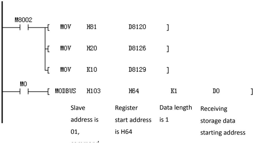
When M0 is set to on, PLC continuously reads the value of register with address of H64 in slave 1, and stores the data in d0 unit.
