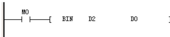
When M0 is ON, the BCD value of D2 is converted into D0 for BIN conversion.
