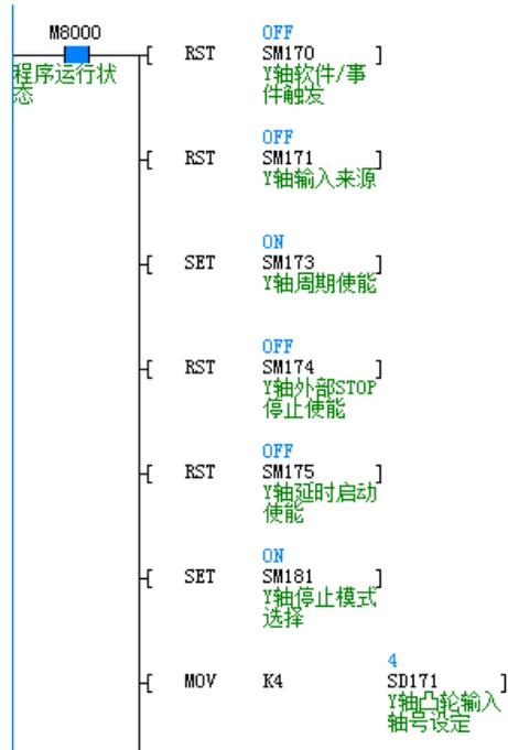
Step 2: Set the flying shear parameters
