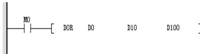
When M0 is ON, D1, D0 and D11, D10 are performed in units of bin or operation result is stored in D101, D100.
