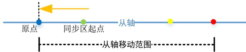
Step 2: Preset the slave axis. After returning to the origin, it is necessary to control the slave axis movement from to the start position of synchronization area, and the start position of the synchronization area is the starting point of the cam engagement.
