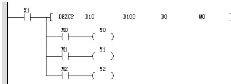
When X1 is ON, (D1, D0) is less than (D11, D10), M0 is ON, and Y0 has an output.
