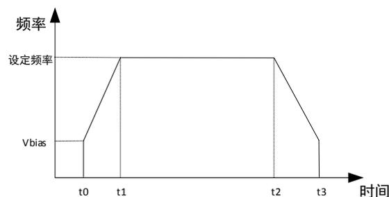
①After the energy flow is enabled, the pulse output frequency will accelerate from the base speed to the set speed according to the set acceleration time (t1-t0). When the output frequency starts to decelerate, it will follow the set deceleration time (t3-t2) and decelerates from set speed to base speed.
