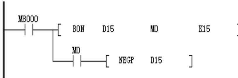
When the 15th bit (bin0-bin15) of D15 is 1 (indicating that D15 is negative), M0 is ON. When M0 is ON, the absolute value of negative D15 can be obtained for D15 Complement.
