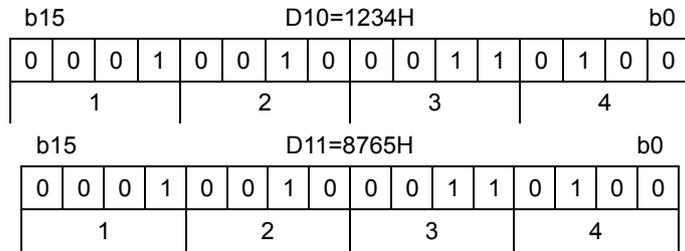
When M8161=OFF, n=4, the composition of the bit is M8161=OFF, n=5, the composition of the bit
