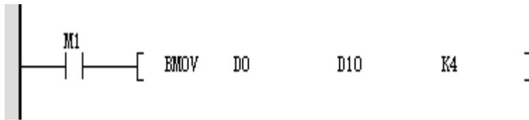
When M1 is on, the value of (D3, D2, D1, D0) is transmitted to (D13, D12, D11, D10).
