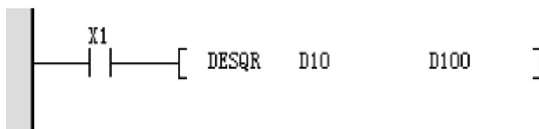
When X1 is ON, the square of the Binary floating number is squared.result  $\sqrt{(D11, D10)}$  , Stored in (D101, D100).
