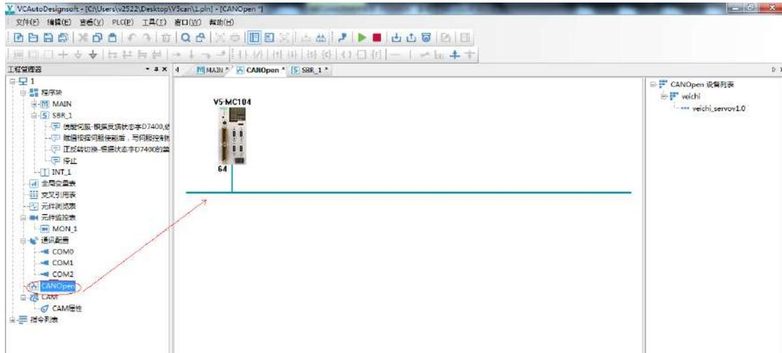
2. Add slave station: double click a device in the "CANopen device list" on the right side of the window to add a slave station, as shown in the following figure:
