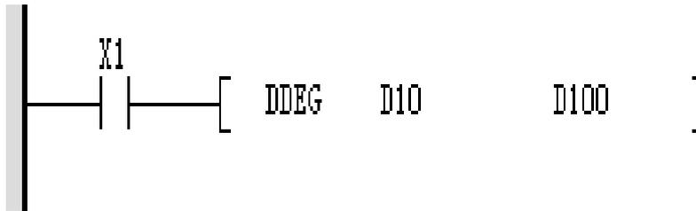
When X1 is ON, the Binary floating number values in (D11, D10) are saved in radians to angles and saved to (D101, D100).
