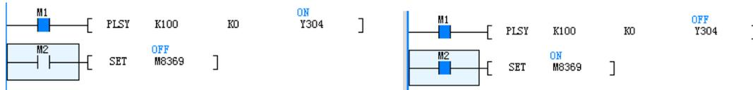
Figure a: before pulse output stop setting
