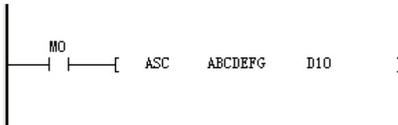
If m8161 = off, after the numeric string is converted into ASCII code, every 2 characters / 1 byte is saved in D in the order of low 8 bits and high 8 bits.
