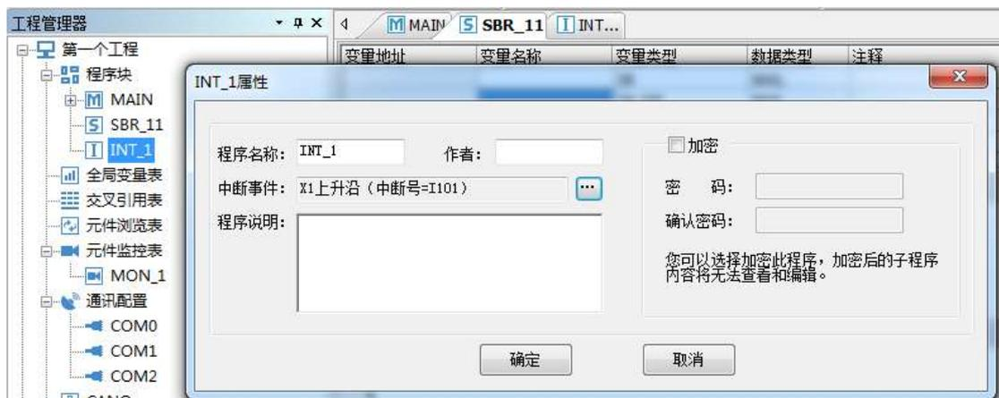
Interrupt Properties Window Click the "OK" button to complete the interrupt settings. The Interrupt Subprogram Properties window allows you to set the program name, author, program description, and encryption.
