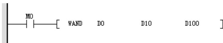
When M0 is ON, D0 and D10 are performed in bin units and the result is stored in D100.
