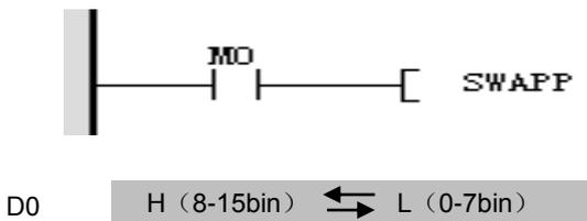
When M0 changes from OFF to ON, the contents of the high byte H and the low byte L in D0 are exchanged.
