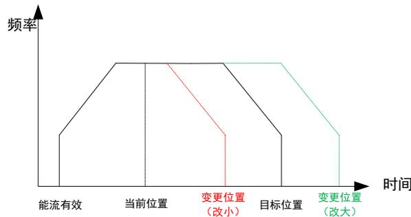
Figure a: the number of modified pulse outputs is greater than the current position
