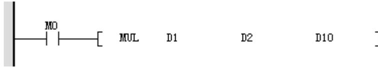
When M0 is ON, the number in D1 is multiplied by D2 and stored in (D11, D10).
