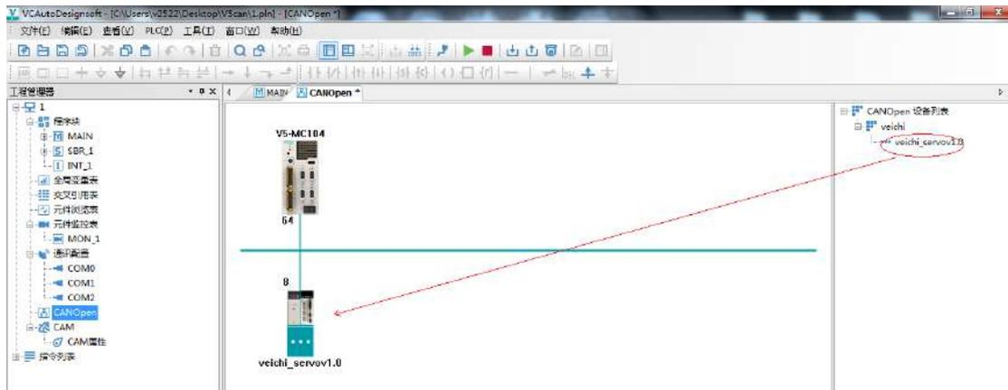
3. Delete slave station: select the slave station in the configuration window, and right-click the pop-up menu to execute "delete" to delete the selected slave station, as shown in the following figure:
