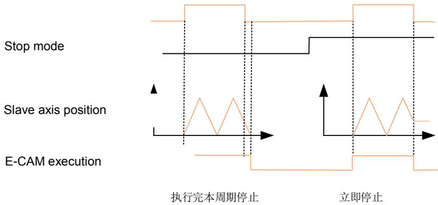
When the stop mode of the E-CAM is set to stop after this cycle is executed, the cam enable position is OFF, the E-CAM will stop after running this cycle, but if the E-CAM execution is needed to stop immediately, the E-CAM running flag can be turned ON to OFF to forced stop the E-CAM.
