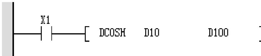
When X1 is ON, the Binary floating number value in (D11, D10) is obtained by taking the COSH value and storing it in (D101, D100).
