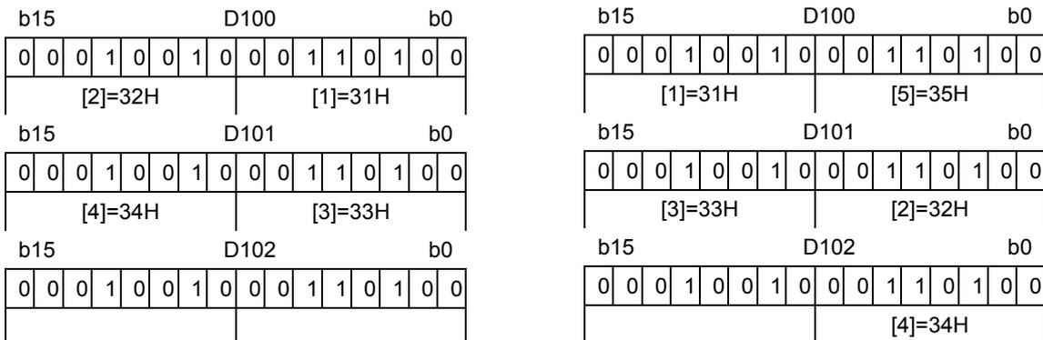
When M8161=ON, n=4, the composition of the bit is M8161=ON, n=5, the composition of the bit
