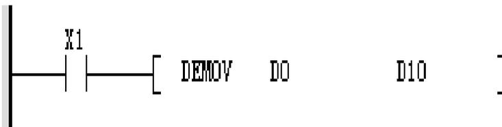
When X1 is ON, the Binary floating number in (D1, D0) is saved to (D11, D10).
