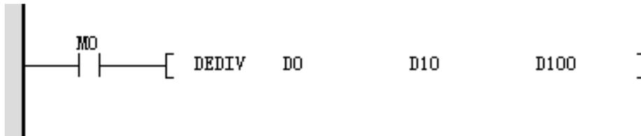
When M0 is ON, the binary floating number (D1, D0) is divided by the binary floating point number (D11, D10), and the binary floating number quotient is stored in (D101, D100).
