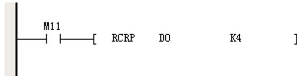
When M11 is on, the number band carry cycle of d0 shifts four bits to the right;
