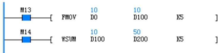
D100~D104 are assigned a value of 10, and M14 is turned ON, and the five D elements starting from D100 address are summed, and the result is stored in (D201, D200).
