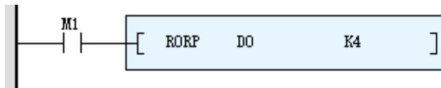
When M1 is on, the number cycle of d0 shifts four bits to the right; The last bit remains in the carry flag bit m8022.
