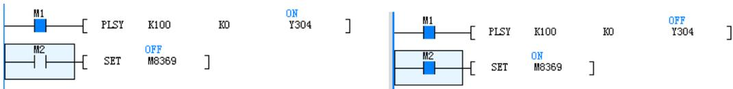
Figure a: Before the pulse-output-stop is set
