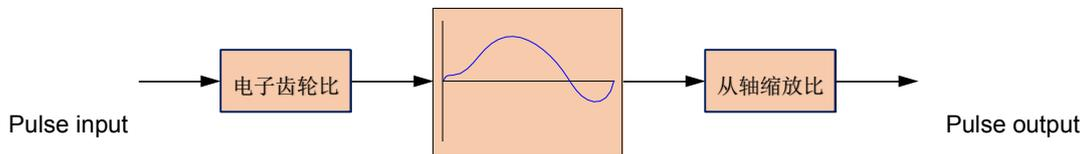
The special components used for the electronic gear ratio and the slave axis scaling ratio are as follows:
