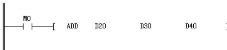
When M0 is ON, the content of D20 plus the content of D30 is placed in D40.
