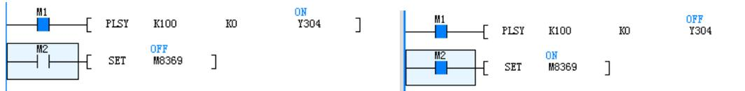
Figure a: Before the pulse-output-stop is set      Figure b: After the pulse-output-stop is set
