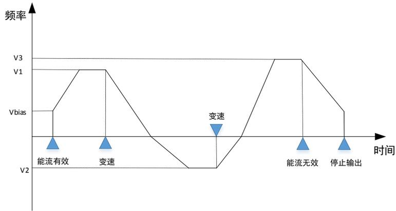
Figure B: plsv2 pulse output change diagram (reverse speed change)
