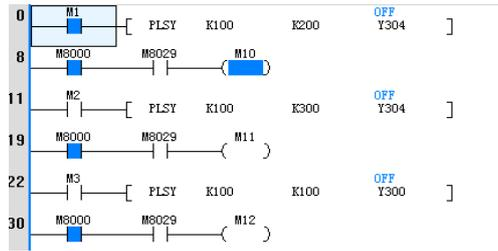
Figure a: M8029 soft components action
