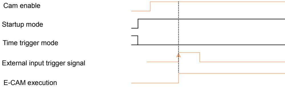
Compare interrupt trigger start timing sequence: (under development)
