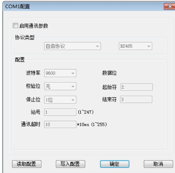
Then select the "enable communication parameters" option, select the "MODBUS-RTU / QLink slave" protocol type, and modify the required "baud rate", "check bit", "stop bit", "station number", "communication timeout" and other parameters. Here, set the slave station number as "2". The interface after Modify is as shown in the figure below. Click the "OK" button to complete the communication settings of the slave station:
