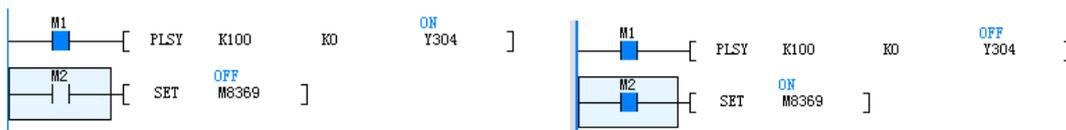
Figure a: Before the pulse-output-stop is set
