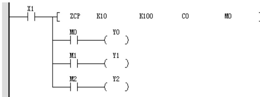
When X1 is ON, CO is less than 10, M0 is ON, and Y0 has an output.
