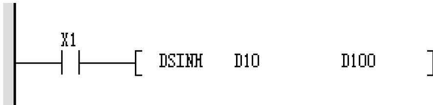
When X1 is ON, the Binary floating number value in (D11, D10) is obtained as the SINH value and stored in (D101, D100).
