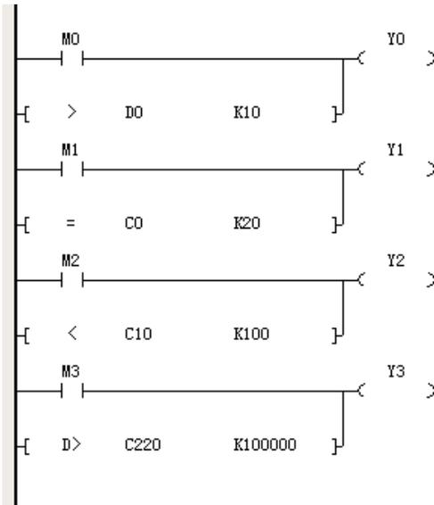
When M0 is ON or the value of D0 is greater than 10, Y0 is ON.
