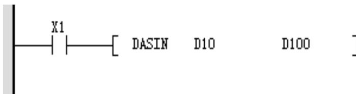
When X1 is ON, the arc (D11, D10) is subjected to the SIN-1 budget and stored in (D101, D100).
