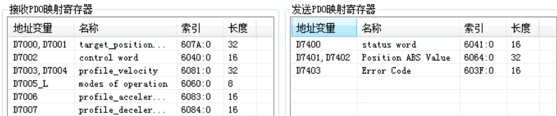
II. When canceling the automatic allocation, you need to enter the address manually. In the added node address table, double-click the D register to be allocated manually, and the mapping register setting interface will pop up. Enter the address to be allocated manually. Note that the address should not be repeated during the manual allocation.
