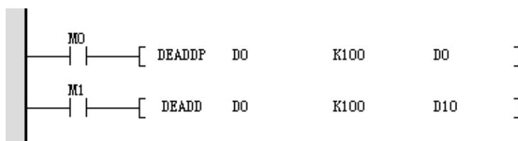
When M0 is ON, the value of D1 and D0 is added to 100 and stored in D1, D0. The constant K100 is automatically adjusted to a binary floating point number before the operation.
