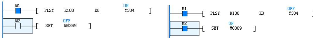
Figure a: before pulse output stop setting
