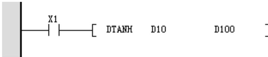
When X1 is ON, the Binary floating number value in (D11, D10) is obtained as a TANH value and stored in (D101, D100).
