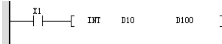
When X1 is ON, the floating number (D11, D10) is rounded and stored in D100.
