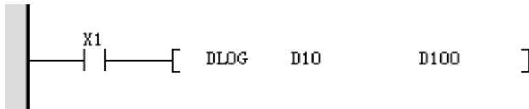
When X1 is ON, the value of Binary floating number in the pair of e (D11, D10) is stored in natural logarithm operation (D101, D100).
