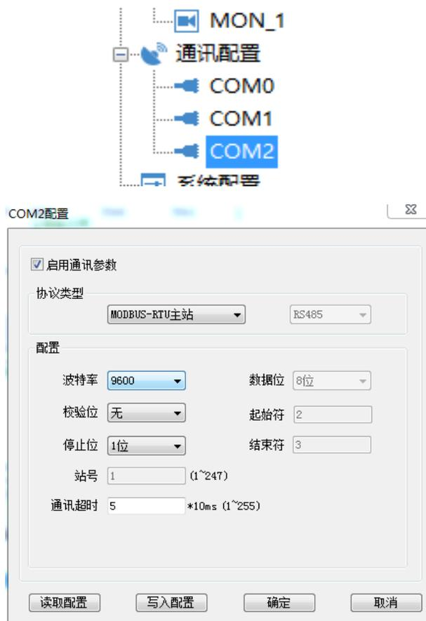
Protocol switching condition: COM2 can switch the protocol when the system is powered on or when the user program is in shutdown state, and the protocol will not be changed in the operation state.
