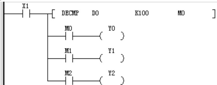
When X1 is ON, (D1, D0) is greater than 100, M0 is ON, and Y0 has an output.
