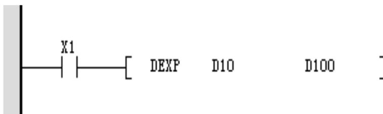
When X1 is ON, the Binary floating number value in the pair e (D11, D10) is indexed and stored in (D101,
