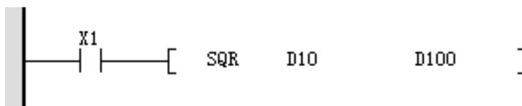
When X1 is ON, the Binary floating number is stored in the D100.
