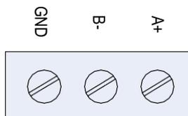
COM1 and other equipment communication connection mode. Through the terminal block, the user can wire on the spot.
