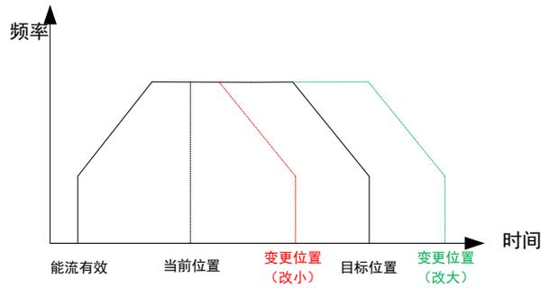
Figure a: The number of modified pulse outputs is more than the current position
