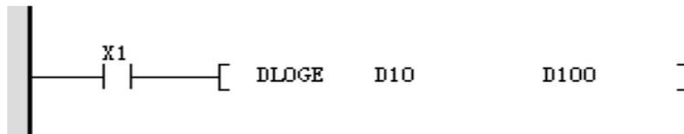
When X1 is ON, the Binary floating number value in the pair e (D11, D10) is subjected to a natural logarithm operation and stored in (D101, D100).
