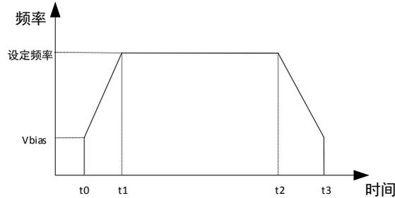
① after enabling the energy flow, the pulse output frequency will accelerate from the base speed to the set speed according to the set acceleration time (t1-t0). When the output frequency starts to decelerate, it will decelerate from the set speed to the base speed according to the set deceleration time (t3-t2).
