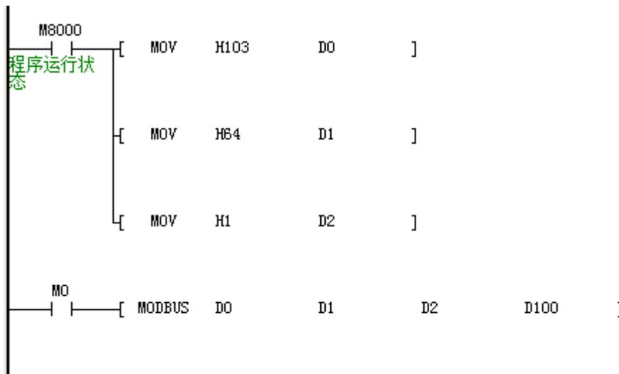
When M0 is ON, read the register with slave address 100 and store it in D100.
