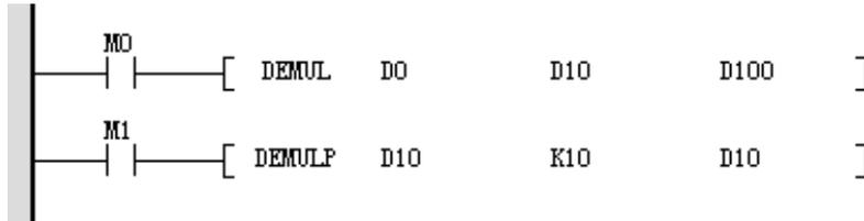
When M0 is ON, the number in D1, D0 is multiplied by D11, and the number in D10 is stored in D101, D100.
